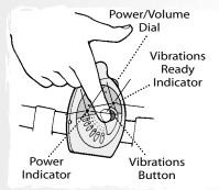
Clip receiver to your clothing (where you will feel vibrations). Walk to the furthest point of use. Rotate receiver power/volume dial to turn power on. Power indicator lights. Now, press the vibrations button. Vibrations ready indicator lights.
